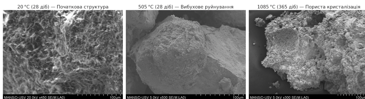
Fig. 1. SEM analysis of high-strength concrete microstructure:
